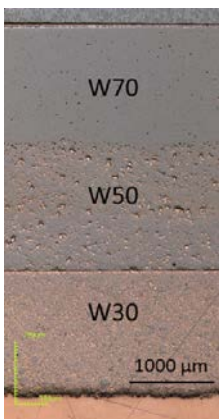
Fig. 24 shows a micrograph of the metallographic section of the W_p/Cu composite interlayer after a HHF test at 20 MW/m 2 (3 cycles) [35].
