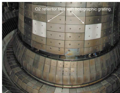
Fig.2 Holographic mirrors for O2 heating mounted on the inner wall of ASDEX Upgrade.
