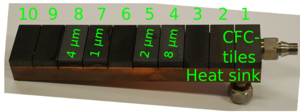
Figure 1: Example of a prototype of the W7-X divertor target element. It consists of 10 CFC tiles (with a thickness of 8 mm, a length of \approx 25 mm and a width of \approx 55 mm) bonded by copper inter-layers to a water-cooled CuCrZr heat sink. The numbers indicated on the tile surfaces denote thickness of the a-C:H surface layers used to emulate real surface layers building up during the W7-X operation.
