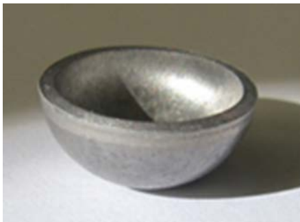
Fig. 16. Heat sink (thimble) of the modular finger target made of tungsten alloy (WL10) which is subjected to pressurized hot helium gas (600 - 700 °C, 100 bar) [39].
