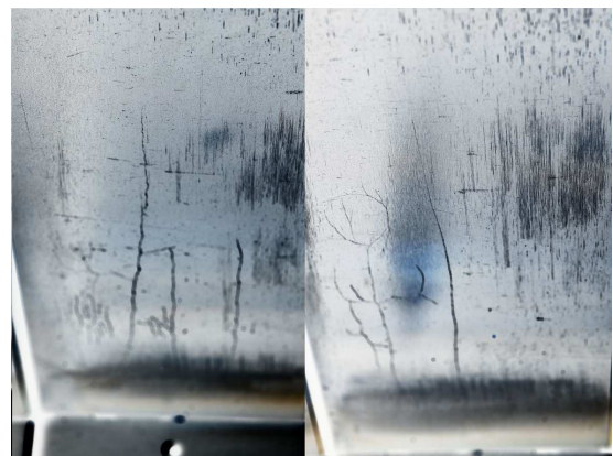
Figure 2: Foto of 2 strike point tiles of the massive W divertor III after 2 campaigns.
