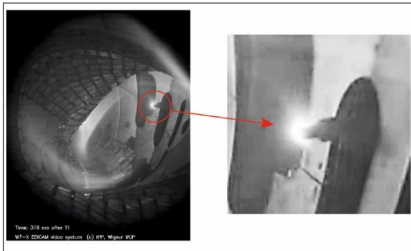
Fig. 6: plasma contact at 275mm stroke depth
